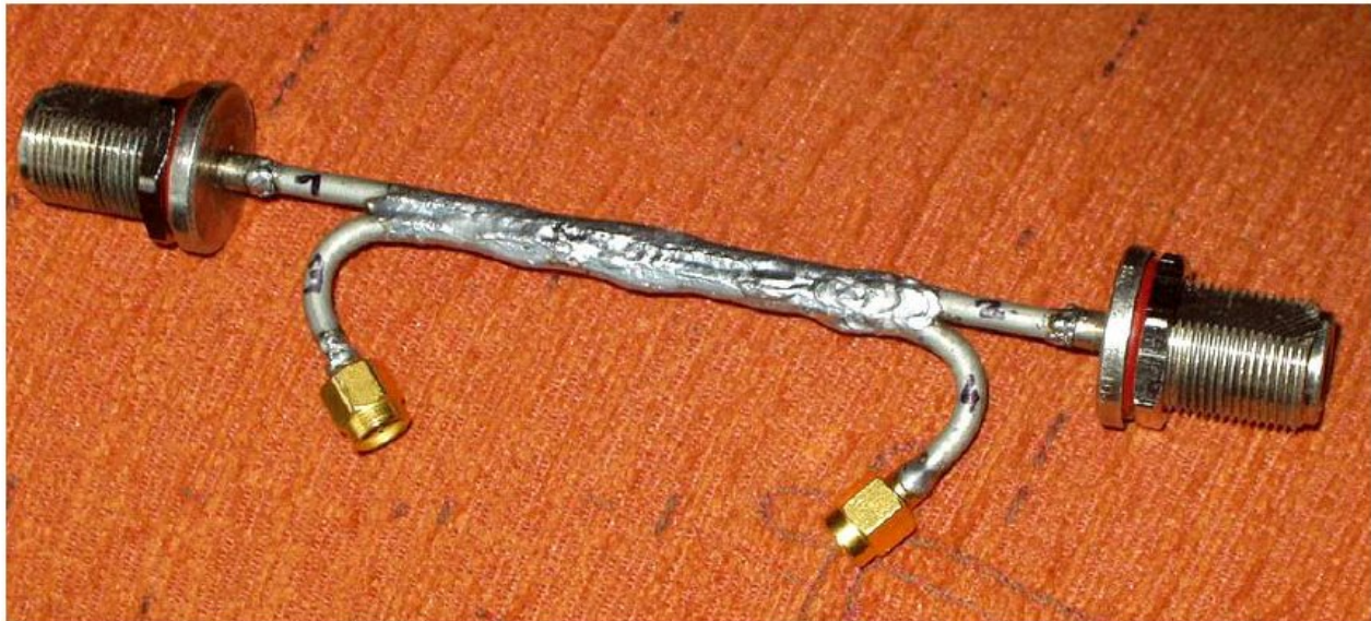
Fig. 2: My construction of the directional coupler
